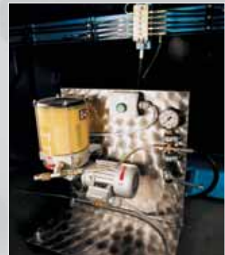
Central lubrication system with progressive distribution
