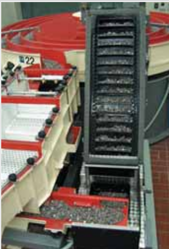
Media conveyor system
