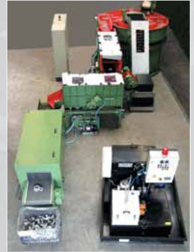
Rotomatic system with part cleaning, drier and process water recycling unit
