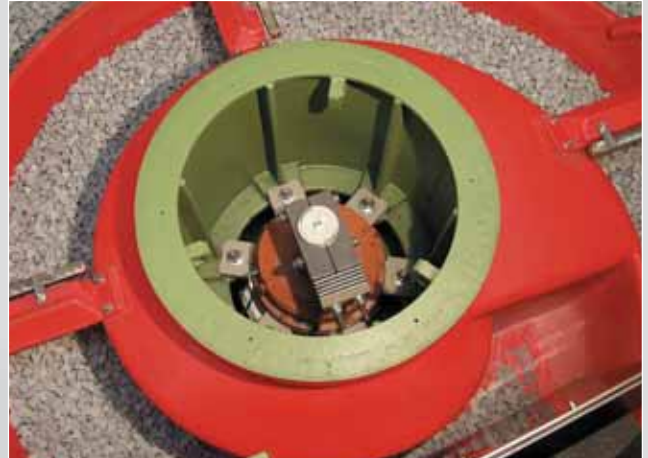
Work bowl with special motor
