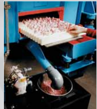
Abrasive media fines separation with collecting zone
