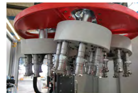
Work piece processing with workstation equipped with eight (8) spindles. Simultaneous processing of 32 work pieces in one batch.
