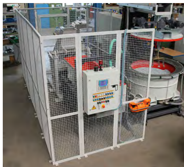
R 4/1300 SF with automatic media replenishment system
