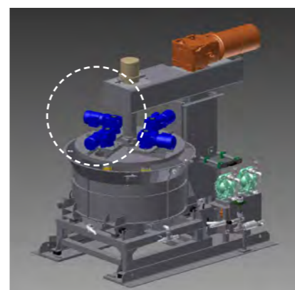
Flexible workstations: Workstation with radial adjustment; maximum work piece diameter up to 600 mm (24") with two (2) work pieces per batch.
