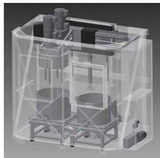
SF - compact drag finisher for 2-stage processing
