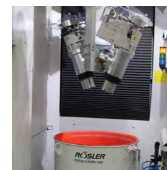
Workstations with servo drive and optional angle and radial adjustment
