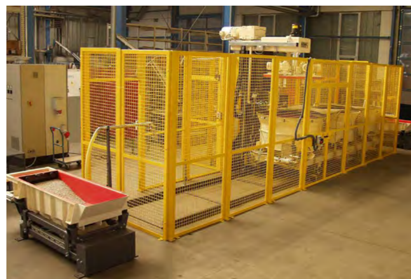
3-station system with automatic media replenishment: Allows cut down, fine grinding and high gloss polishing without having to remove the work pieces from the workstations.
