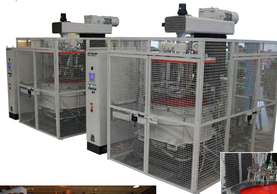
3-station system with automatic media replenishment: Allows cut down, fine grinding and high gloss polishing without having to remove the work pieces from the workstations.
