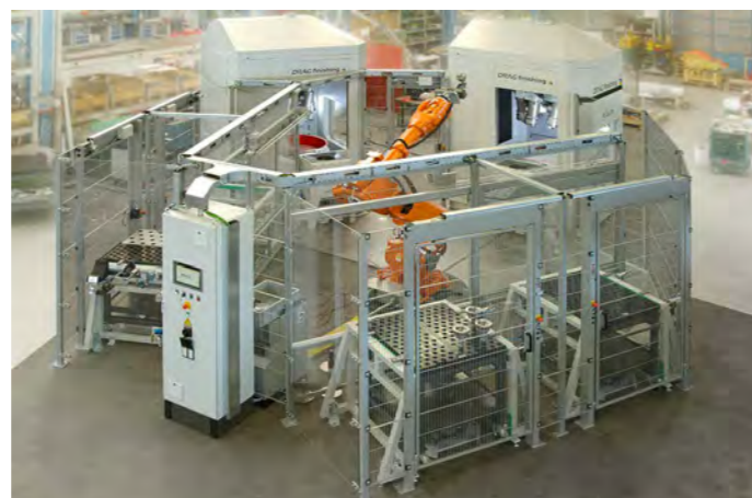
R 6/1000 "SF-A" with robotic work piece handling (complete production center)
