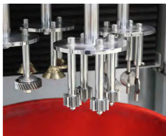
Fixtures for placing multiple work pieces on a spindle without angle adjustment.
