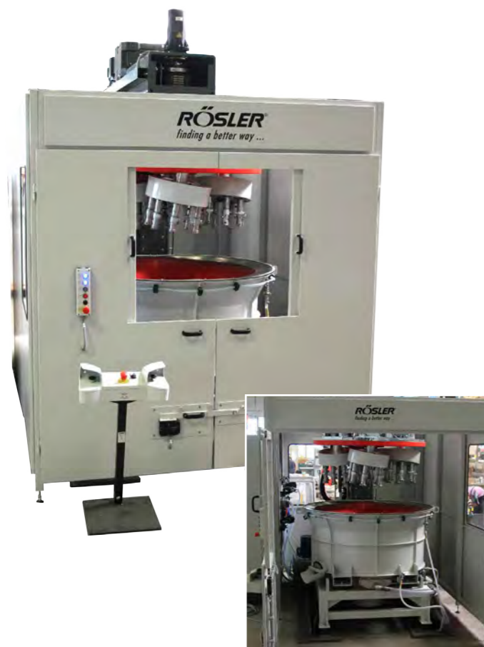
Drag finisher with protective cabin: High work place safety combined with noise reduction.
