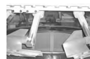
Maxi drag system for big, heavy work pieces
